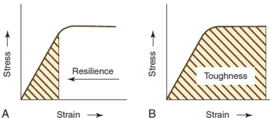
FIG 2-6 Stress-strain curves illustrating the areas that give a measure of the resilience (A) and toughness (B).
